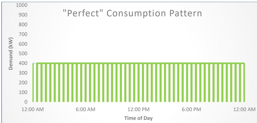
While this is great in theory, it isn't actually possible as industrial processes make use of a variety of equipment, at varying times and each with its own power requirement. Fortunately, while controlling loads to eliminate peaks in demand may be very difficult, there is another solution to reduce your demand.
