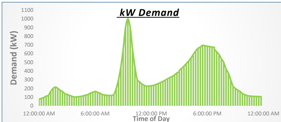
The above graph shows how a company may consume energy on a typical day. Here two major peaks are noted at 1000 kW and 700kW. Even though the 1000 kW peak is sustained for only about one hour, this company's demand charge will be based on this highest peak for the entire month, regardless if it occurs daily or once per month.
